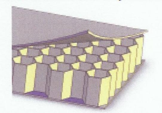
The weight of the spacecraft structure is minimized by using honeycomb aluminum panels. The 1" thick panels are made of 1/8" cell aluminum honeycomb core with 0.005" thick aluminum foil sheets bonded to each face. This design cuts the weight of each panel to 1/9 that of an equally strong solid aluminum panel.
