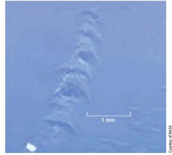
This image was captured by the orbital debris collector experiment flown on the Russian space station Mir. The experiment was delivered and retrieved by NASA space shuttles STS-76 and STS-86. The collector used an aerogel—a very low-density material sometimes called "solid smoke"—to slow and capture the particles. The space debris shown in this image is a paint flake. In 1994, a paint flake about this size created a crater almost 1/2 inch in diameter in a shuttle side hatch window.
