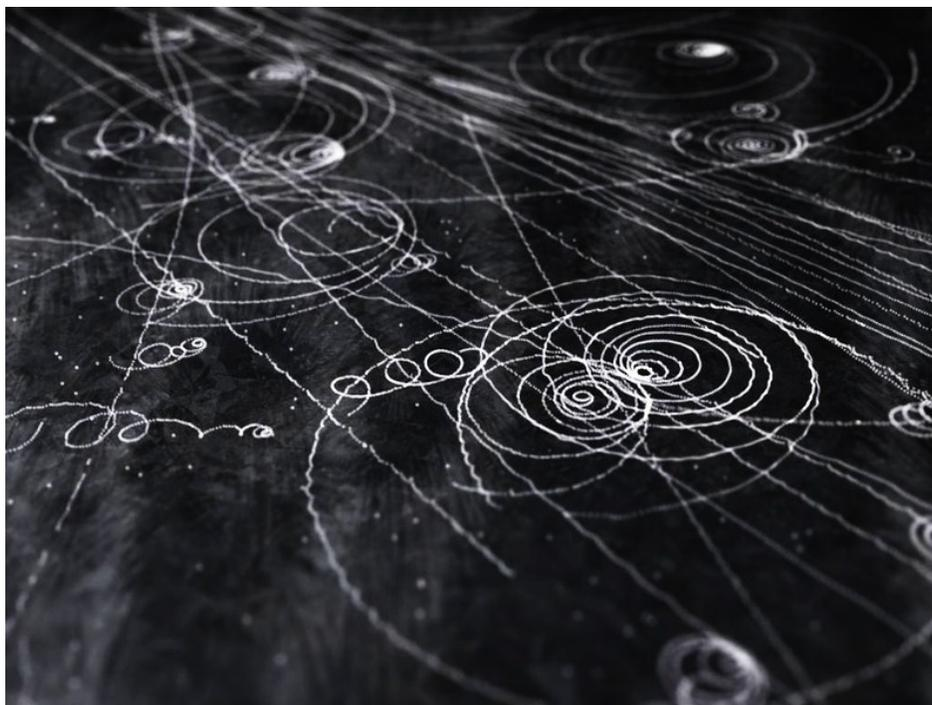
Which particles can be seen in the cloud chamber? Since the principle of operation is based on the ionization caused by the passage of the particle, it results that the higher the ionization capacity and the greater the visibility of the trace.
