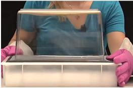
7. Wait a few moments while the warm IPA (It is very volatile, molecules move quickly, so there's lots of energy and heat in the IPA) is evaporting into the chamber. It settles down towrd the dry ice and condences. Any disturbance in the air from these moving molecules will create a cloud.
