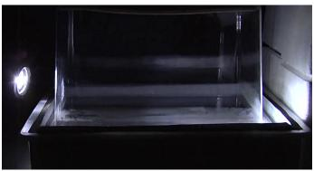
8. Swith off the lights and use a strong light source shining from the side of the chamber.
